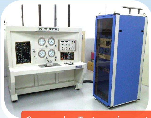
Servo valve Test equipment
